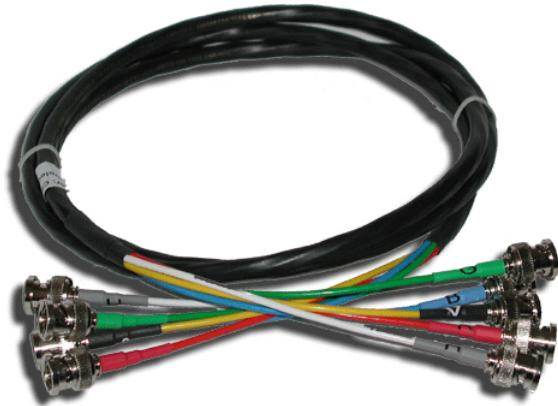
Kramer's CP-5BM/5BM series cables are constructed of plenum rated 5 mini coax cables in a single jacket with BNC 75Ω connectors at each end. They offer outstanding quality, durability, and high performance for any RGBHV video signal application where a plenum rating is required
